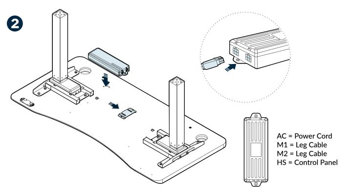
Once the legs are secured with screws and while the desk is still face down, lower the control box onto the control box bracket and slide it to engage it securely in place. When the control box is secured, connect the leg cables to the corresponding control box inputs, M1 and M2.
