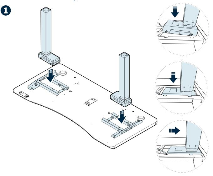
Desktop and desk legs will arrive in separate boxes. We recommend assembling the desk with the desktop face down in its box to prevent any surface scratching. Open both boxes; remove the desk legs and parts from their box.
