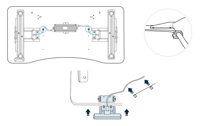
Locate the control panel and slide it into the bracket to attach. Once the panel is in place, connect its cable to the corresponding control box input, HS.
