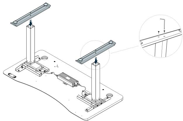
Once the control box is secure and while the desk is still face down, place one foot on top of one leg aligning the screw holes. Use the larger hex key (M10) provided to securely tighten screws (M10 - 40mm) into the feet. Repeat this step to attach the other foot.
